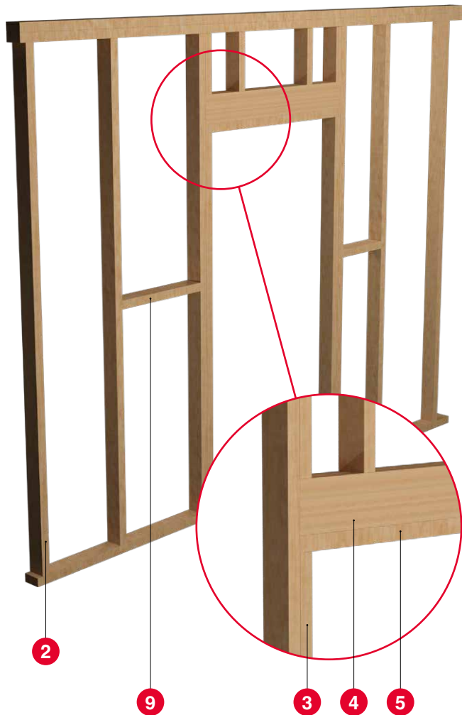
View 1 – external wall structure with door opening
