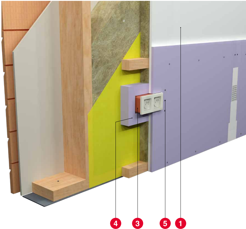
View 1 – Electrical sockets in the external wall
