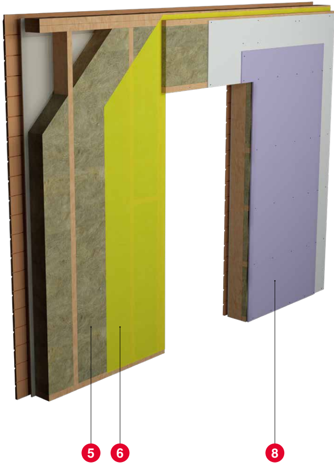
View 3 – wall structure with a door opening with internal cladding – view from the interior
