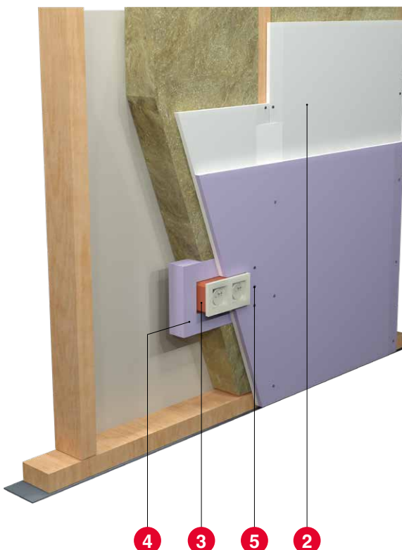
View 2 – Electrical sockets in the partition wall
