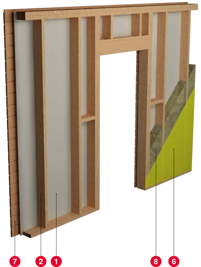
View 2 – external wall structure with door opening with facade – view from the room side
