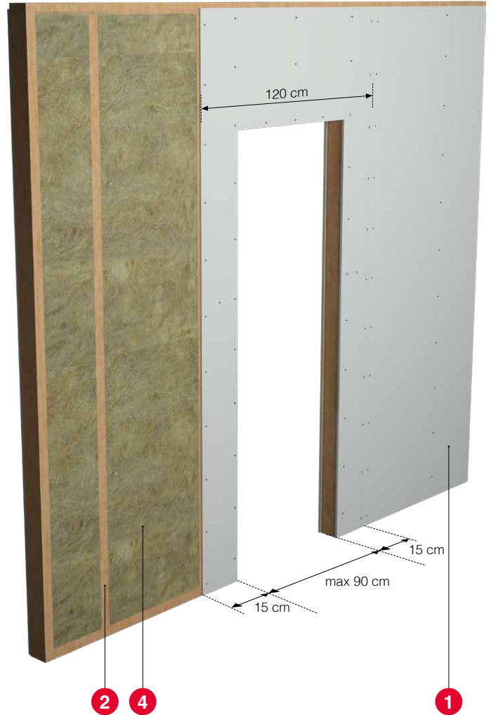
View 2 – partition wall structure with door opening – 1 crossbar – lining
