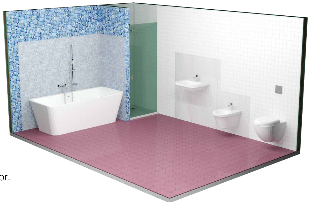
Fig. 37. Wall areas particularly exposed to water splashes in a bathroom (marked grey)
